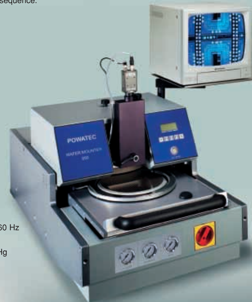
Push sliding table into mounting position and withdraw again. Chuck is now ready for another wafer and frame, i.e. the next sequence.
