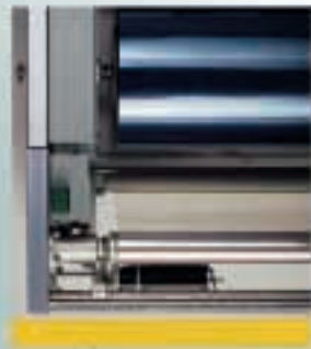
Protective foil, automatically wound up
